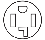
4-wire receptacle (14-30R)
